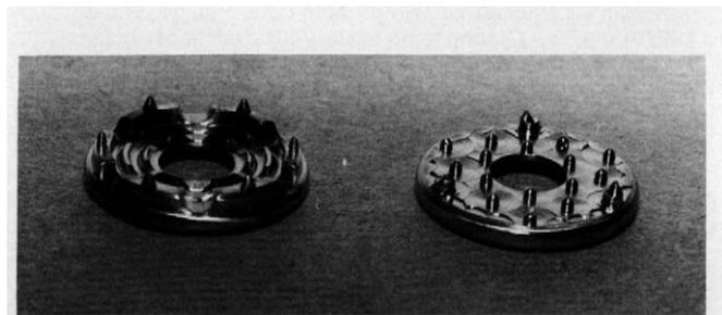
**Figure 1.** The two prototypal washer designs (16-mm diameter) used in the mechanical tests.
