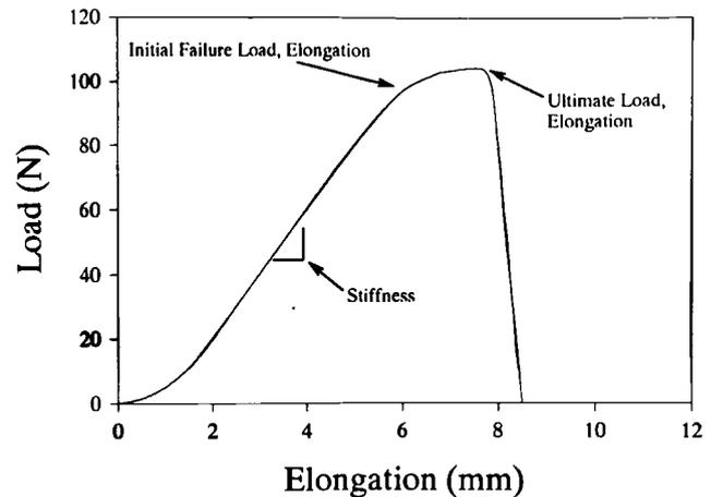
**Figure 4.** A representative load-elongation curve of a femur-washer-fascia lata complex shows how the various structural parameters were defined.
