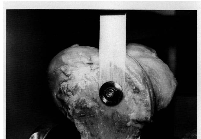
**Figure 5.** Mode of failure for fascia lata fixation. In all cases the fascia lata shredded from beneath the fixation device.
