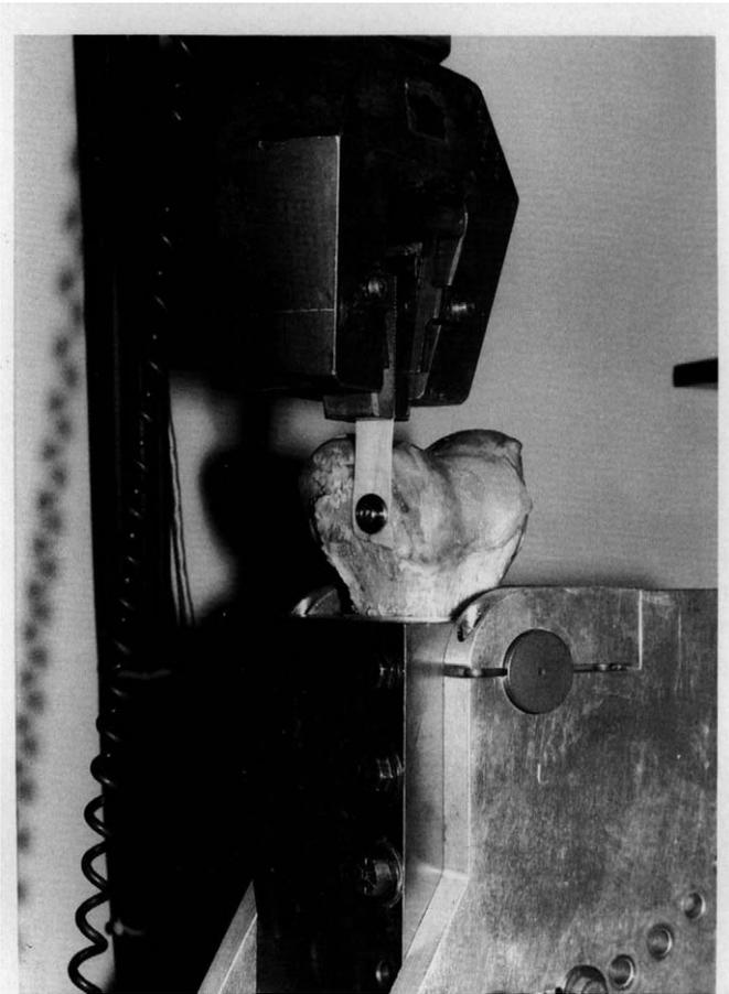
**Figure 3.** The test setup used for evaluation of the structural properties of the femur-washer-fascia lata complex.
