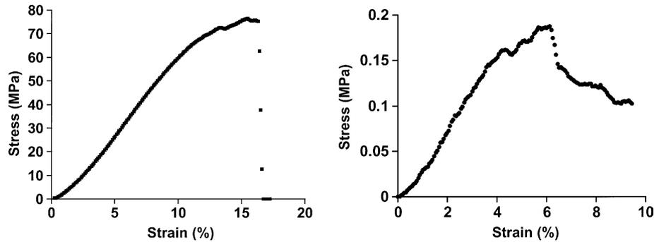
Fig. 4. Typical stress–strain curves from longitudinal (left) and transverse (right) specimens taken from the same IOL. Note the differences in stress and strain scales.
