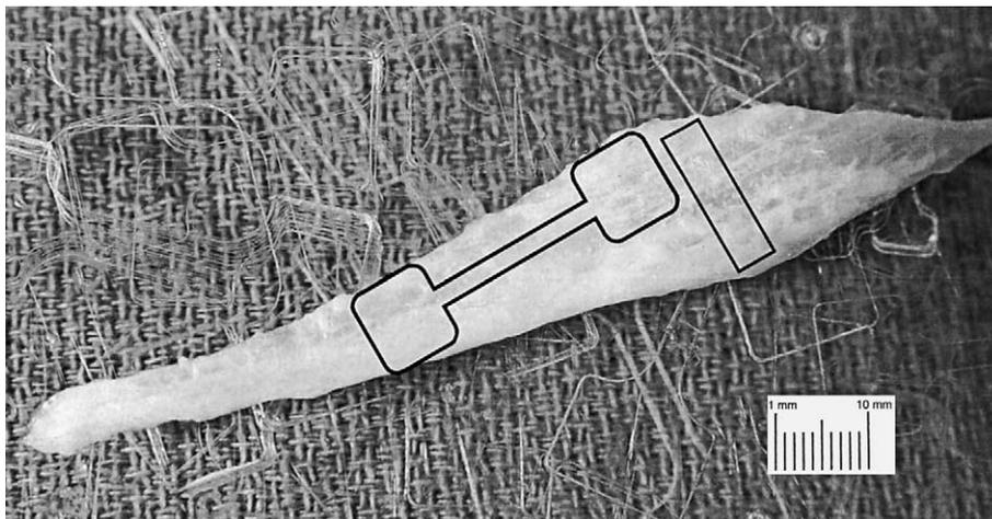
Fig. 2. Midsubstance of an IOL after excision from a cadaveric forearm with schematic showing how typical dog bone (longitudinal) and rectangular (transverse) tensile test specimens were taken.
