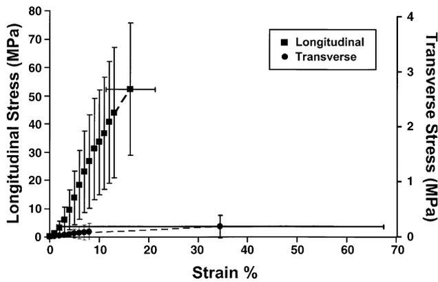
Fig. 5. Average stress–strain curves for 20 human IOL longitudinal and transverse specimens. Note the difference in stress scales (left: longitudinal; right: transverse).
