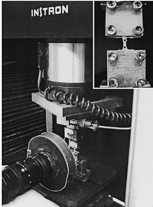
Fig. 3. Photograph of the tensile test set-up showing the video camera and a close-up view of the strain markers taken just prior to initiation of the preconditioning and load to failure protocol.
