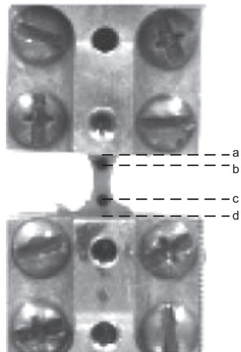
**Fig. 2.** Specimen sample positioned for testing within the MTS. The upper and lower clamps hold the tabs of the dog bone-shaped sample. Black markers, visible in the camera images, were affixed to the central portion of the sample as b and c in the figure. a: upper clamp edge; and d: lower clamp edge.
