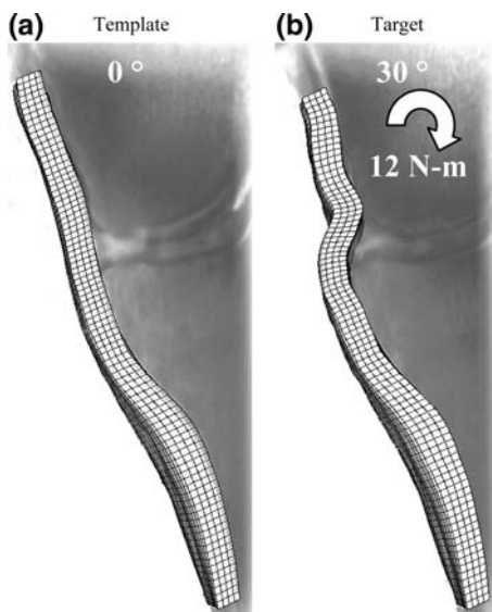
FIGURE 4. Hyperelastic Warping solution for knee 1, showing side view of the original and deformed FE mesh superimposed on volumetric MR images of the template and target, respectively. (a) Template with knee at 0° flexion; (b) Deformed template for knee at 30° flexion with 12 N m valgus torque.
