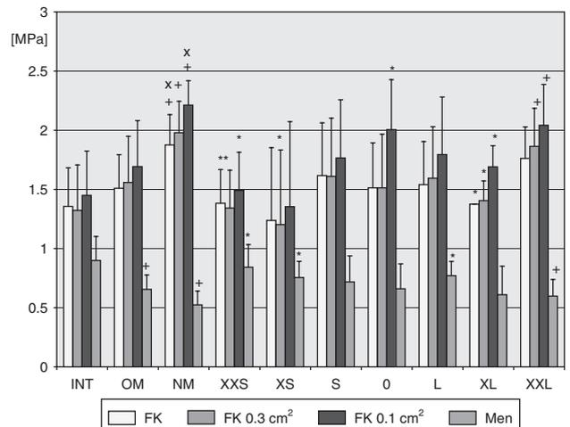
**Figure 10.** Contact pressures for the intact knees (INT), knees with the replanted original meniscus (OM), and knee after meniscectomy (NM) and for the different allograft groups after allocation from the mean of their inner diameters in extension.  $*p_{NM} < .05$ .  $+p_{INT} < .05$ .  $xp_{INT} < .05$ . Linear regression analysis:  $p_{PFK0.3cm^2} = .044$ ;  $p_{PFK0.1cm^2} = .033$ ;  $p_{PMen} = .039$ . See text for complete description of abbreviations.
