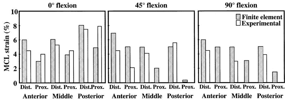
**FIGURE 15.** Comparison of experimental and FE MCL strains with 5 degrees of applied valgus rotation. Ligament buckling prevented experimental measurements in the proximal region at 45 and 90 degrees.
