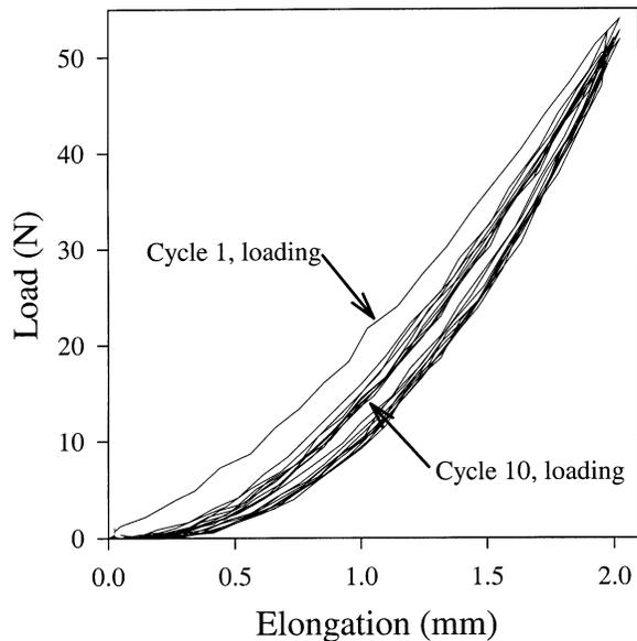
**FIGURE 8.** Cyclic load-elongation behavior of human fascia lata tested along the collagen fiber direction. The hysteresis decreases with increasing cycle number, and the loading-unloading curves become repeatable. (Reproduced with permission from Weiss et al., 1996.)
