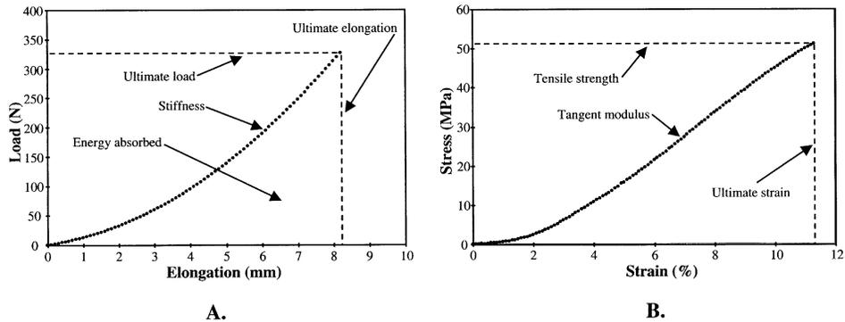
**FIGURE 6.** Load-elongation and stress-strain curves for a bone-ligament-bone complex under uniaxial tension. (A) Structural properties represented in a load-elongation curve, (B) Material properties represented in a stress-strain curve.
