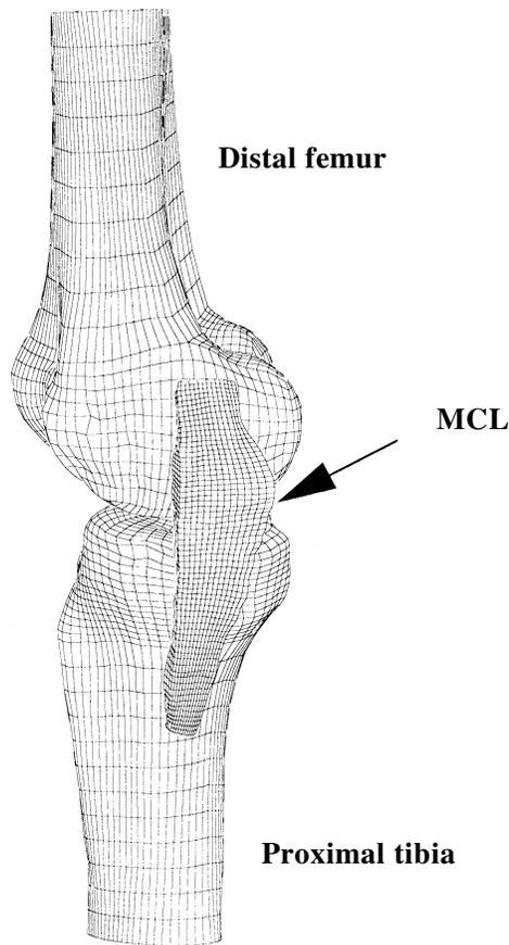
**FIGURE12.** FE mesh of the femur-MCL-tibia complex. The bones were represented as rigid and the MCL was modeled as a transversely isotropic, hyperelastic material. Experimentally measured kinematics were used to drive the model.
