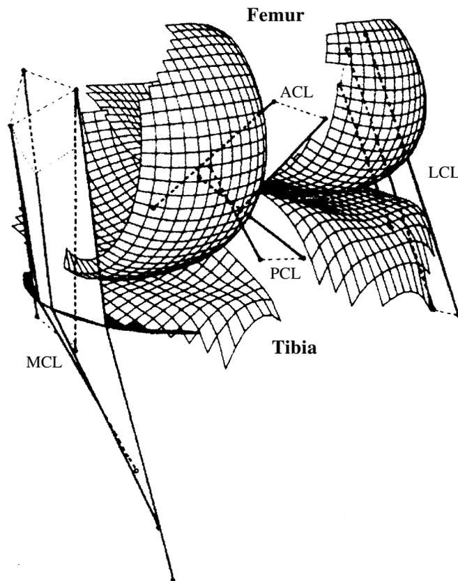
**FIGURE 11.** FE model of the human knee joint featuring a discrete element representation of the ligaments. An algorithm has been used that allows for wrapping of the MCL around the medial edge of the tibia. (Adapted from Blankevoort and Huiskes, 1991.)
