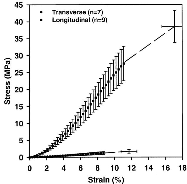
**FIGURE 7.** Stress-strain curves for human MCL tested parallel and transverse to the collagen fiber direction. The final point in each curve was the average failure point for the specimens. The error bars indicate the standard error for the average ultimate strain and tensile stress. The tangent modulus of the longitudinal curve was over an order of magnitude greater than the tangent modulus of the transverse curve. (Reprinted with permission from Quapp and Weiss, 1998.)
