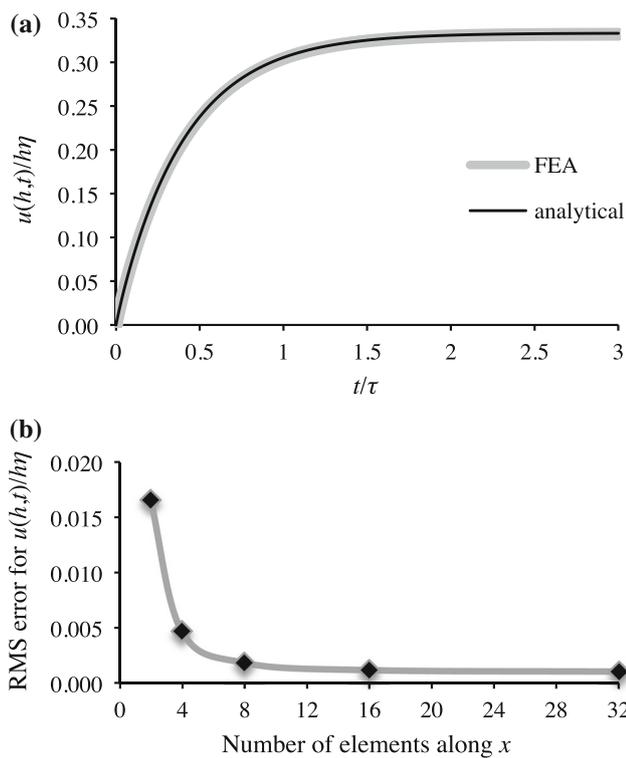
**Fig. 4** **a** Surface displacement  $u(h, t)/h\xi$  for 1D analysis of interstitial solid growth. The analytical solution is based on (59), with  $\eta = (1 - \varphi_r^s) \hat{\zeta} \bar{\nu} \tau$ . The finite element solution was obtained using  $h = 1$ ,  $H_A = 1$ ,  $k = 1$ , and  $(1 - \varphi_r^s) \hat{\zeta} \bar{\nu} = 10^{-3}$ . **b** Mesh convergence results
