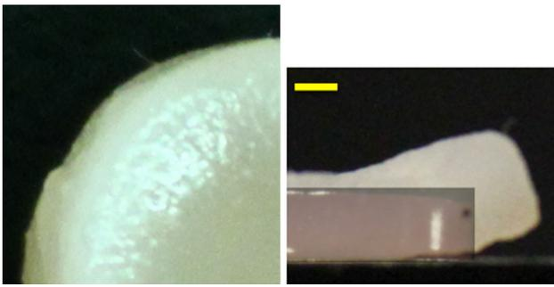
**Fig. 6** Cartilage construct engineered from chondrocyte-seeded agarose gels. Side view of construct at right shows an overlay of a day 0 construct over the image of the day 53 construct. The increased bulging and construct opacity at the outer periphery is qualitatively consistent with the shape and matrix deposition distribution of the finite element results in Fig. 5 (Scale bar 1 mm)
