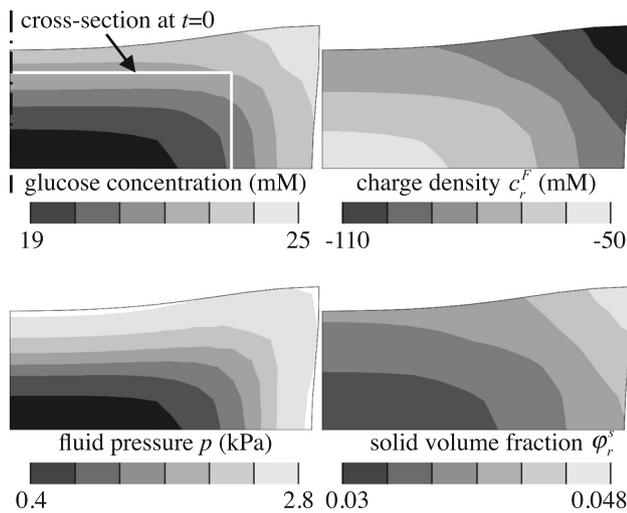
**Fig. 5** Axisymmetric analysis of engineered cartilage growth with glucose consumption and synthesis of negatively charged CS. The tissue construct, which is initially cylindrical, rests on the impermeable bottom of the culture dish. This cross-sectional view shows an outline of the construct and contour maps of the glucose concentration,  $c_r^F$ ,  $p$  and  $\varphi_r^s$  at day 30
