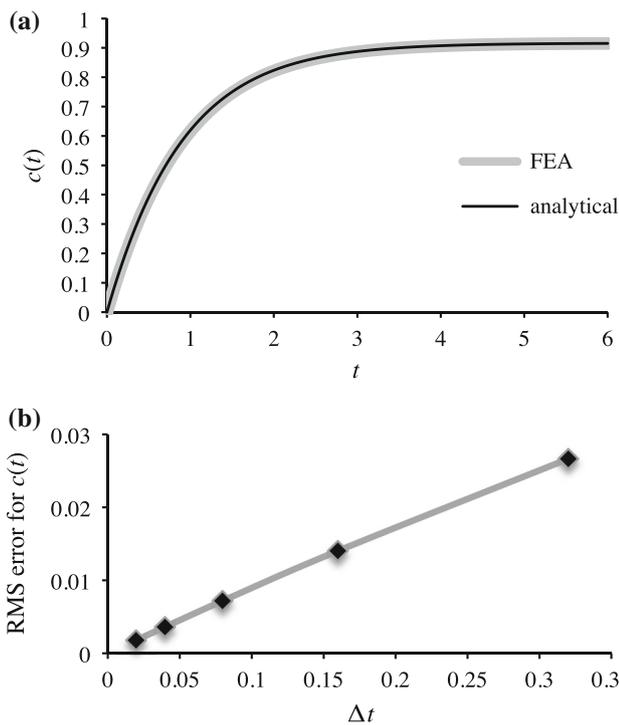
**Fig. 1** **a** Time-dependent dissociation of NaCl into Na<sup>+</sup> and Cl<sup>-</sup>. The ion concentration  $c(t)$  was evaluated from a finite element analysis and from the analytical solution of (53), with  $c_t = 1$ ,  $k_f = 1$ , and  $K_a = 10$ . **b** Time discretization error analysis
